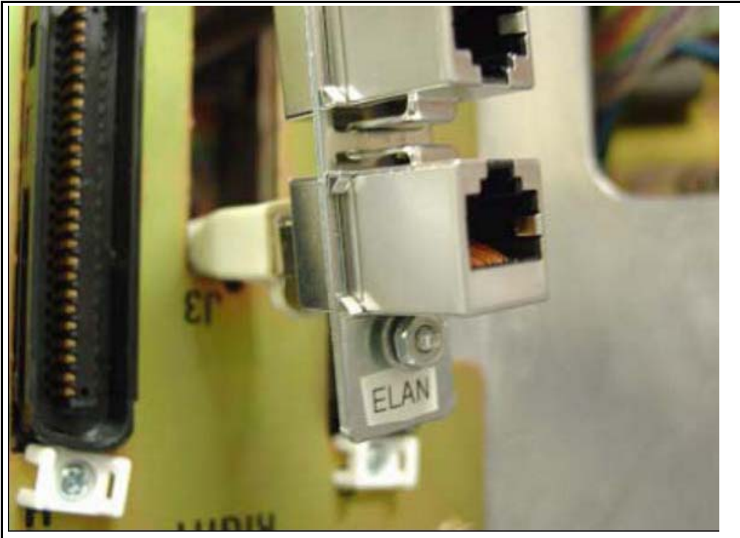
Figure 35 ELAN connection on Ethernet port coupler
